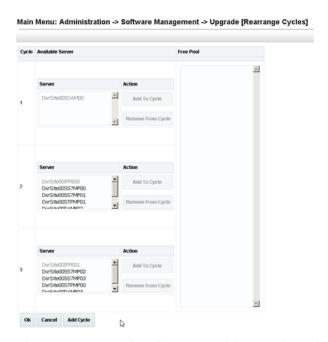
3. When a server needs to be removed from cycle and needs to be added in an existing cycle or a new cycle, select the desired server in the list and click **Remove from Cycle**. The server moves to the Free Pool on the right side.
